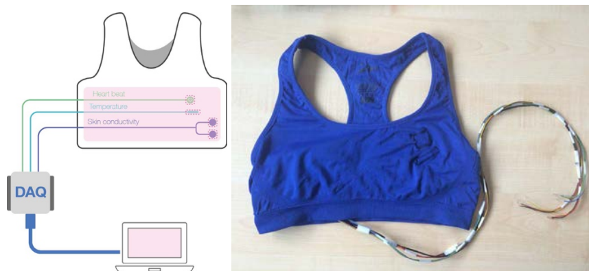
Figure 2: Connection of electronics and placement of sensors of Prototype 1
