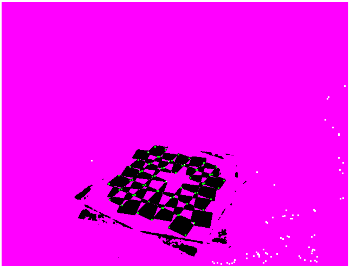
Figure 6.12: The result of Shi Tomasi feature detector (Figure 6.8) was superimposed onto the binarised image. The background features lying at the white region were subsequently removed.
