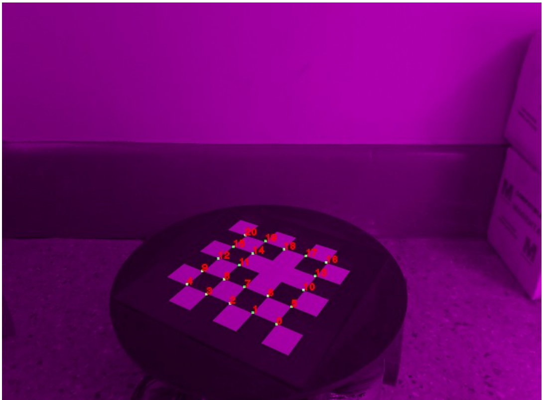
Figure 6.14: Image showing the detected salient features. All the detected twenty one X-corners are highlighted in yellow.
