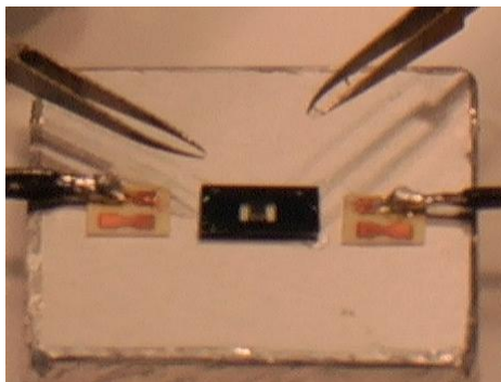
Figure 46: Micro soldering workstation with two SSSA grippers in view
