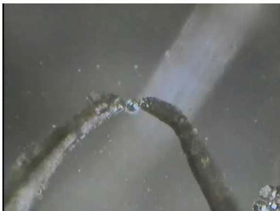
Figure 48: SSSA gripper grasping a solder sphere
