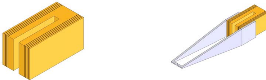
Figure 6: Normally closed gripper actuator (left). Gripper arms are assembled to the piezoactuator to magnify the stroke (right).
