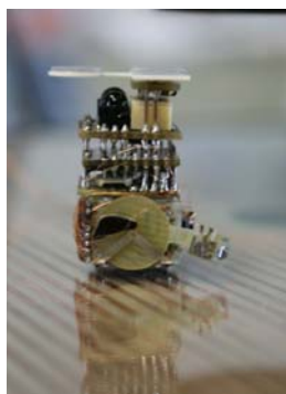
Figure 53: Single MICRoN robot with integrated SyringeChip (real robot and 3-D-Simulation).
