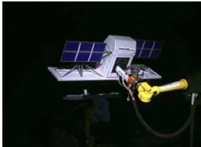
Figure 7: Robot Mounted Satellite Model of a Radarsat satellite was mounted on a 6 dof articulated
