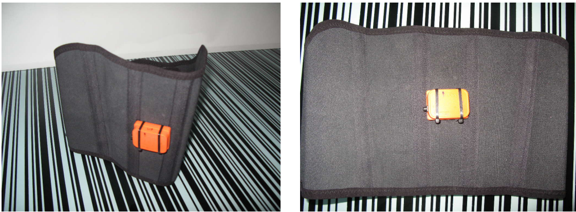
Figure 3.2: IMU XSens MTx device on a back rubber band
