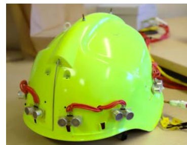
Figure 1: Early prototype device to aid mobility for the visually impaired
